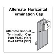
The FPI AstroCap XL<sup>™</sup> is certified for installations using FPI venting systems as well as Simpson Dura-Vent® and Direct Vent GS.
